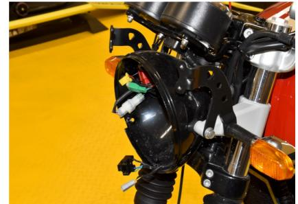
Locate the vehicle speed sensor connectors.
